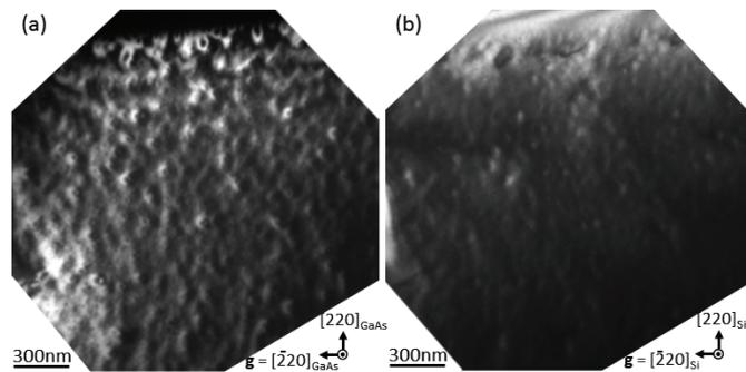
Fig. 1. Plane-view TEM images of a Si/GaAs interface fabricated by SAB at room temperature, taken with the reflections of  $\mathbf{g} = [220]$  (a) for GaAs and (b) for Si. We can select those reflections separately due to an off-angle of  $5^\circ$  on the (001) surface of the GaAs substrate.
